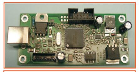
The USB Interface connects a PC with a Braille Line assembled with metec Braille Modules (B11 or B16) This Doku is valid for the USB-Device 01#00.
